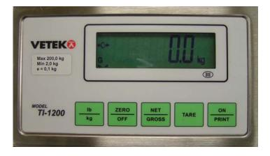
All Scales are EC type-approved non-automatic weighing instrument Accuracy class III Basically, the Weighing Indicator (TI-1200-S), is the same in all Scales.
